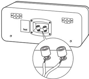
Use the connection terminal with the two clamps on the back of the speaker to connect the speaker cables. The terminals are each marked red (+) and black (-).
