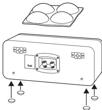
If you would like to set the speaker up, attach the 4 enclosed rubber feet to the corners of the speaker base. As a result, interference due to vibrations is avoided.
